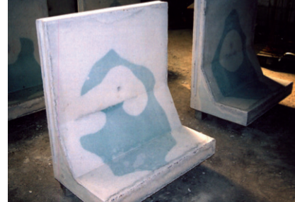
FIGURE 1 - Blue-green colouring observed on concrete containing slag (left, ready-to-use concrete; right, prefabricated concrete - © Eqiom)
